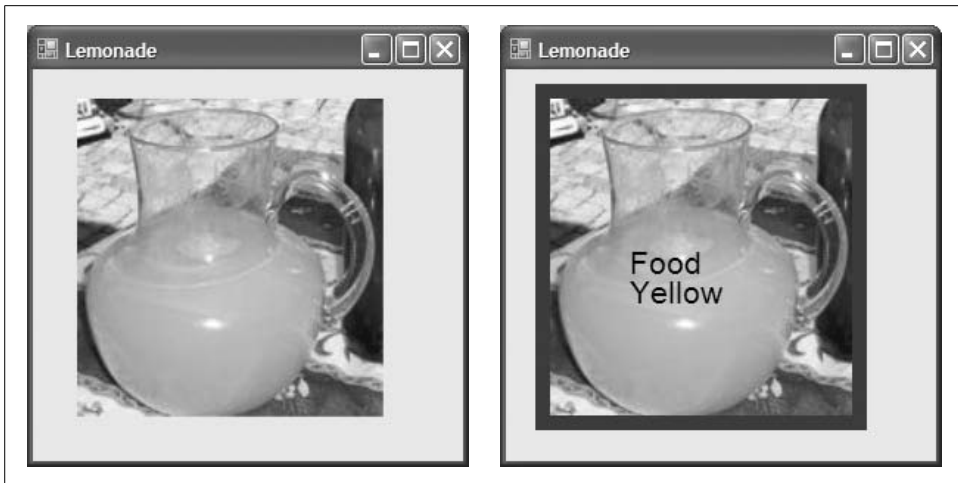
Figure 2-1. Decorator pattern illustration—(a) plain photograph and (b) photograph with tags
